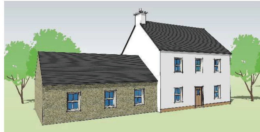
Figure 5.19 – Appropriate use of stone as a wall finish on all elevations of the side annex.
