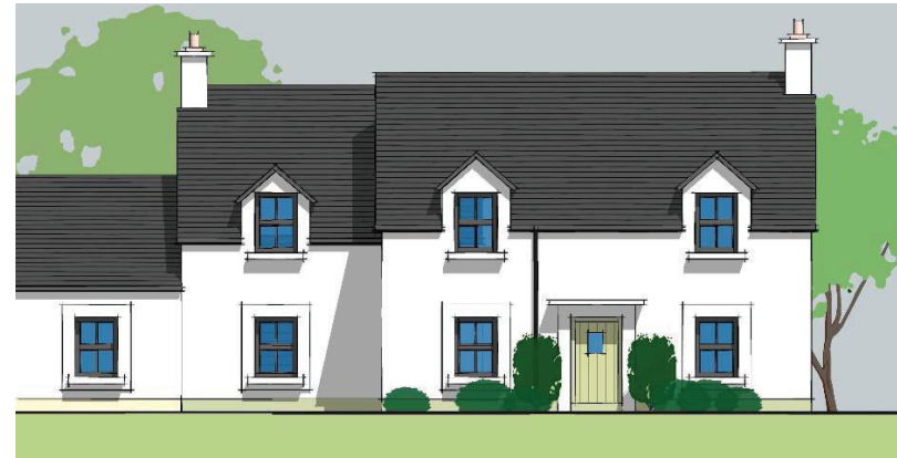
Figure 5.8 – Simple interpretation of a dormer building form with dormers on the front elevation projecting from the main wall.
