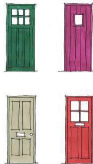
Figure 5.13 – Appropriate simple design vertical sheeted doors.
