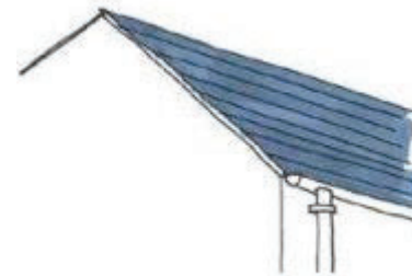
Figure 5.2 – Appropriate minimal roof edge treatment
