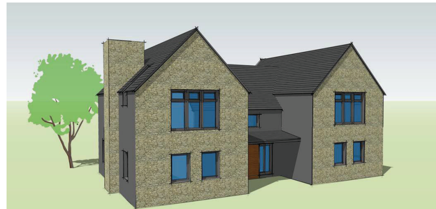
Figure 5.20 – The application of stone on projecting front gables only is less successful visually.
