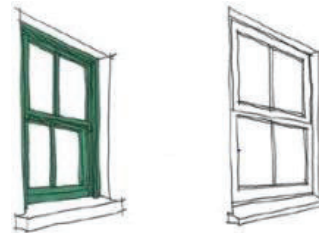
Figure 5.12 – Timber window and uPVC window.
