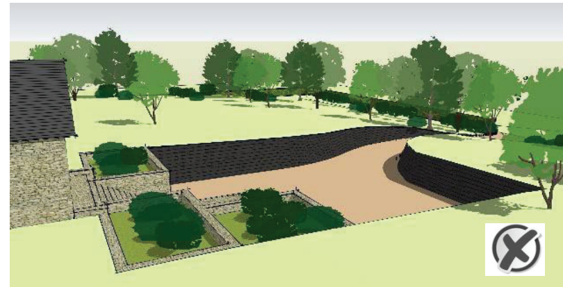
Figure 3.5 - Example of excessive cutting to facilitate driveway.
